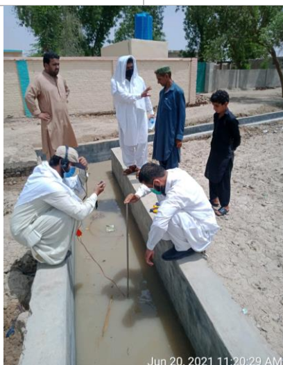
Figure-4.148: Checking Water flow using Pygmy Meter
