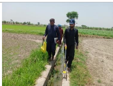
Figure-4.86: Measuring the length of watercourse with measuring wheel of Watercourse 125800/R
